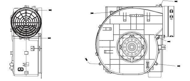
4. loosen the nut fixed on the motor shaft, remove the nut, pull out the exhaust air wheel with both hands; remove the 4 screws fixed on the other side, remove the motor
