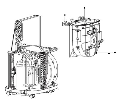
2. remove the WIFI components fixed in the duct volute with two screws and five volute screws.
